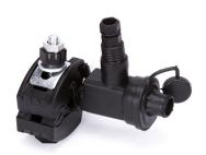
Main line cross-section:6-95 mm²Main line diameter:3.05-12.5 mmBranch line cross-section:1x(16-95) mm²Branch line diameter:7.0-15.7 mm
